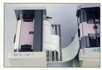
**Optional Interstacker** – With Duplo's optional interstacker, side-by-side forms can be slit and stacked sequentially (for V-760 only).
